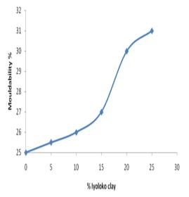
Figure 5, Variation of Mouldability with % Iyoloko clay
