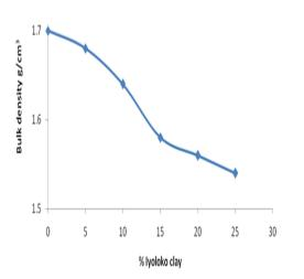
Figure 2, Variation of Bulk Density with % of Iyoloko clay
