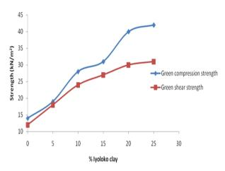
Figure 6, Variation of Green Strength with % of Iyoloko clay
